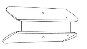
2. Gently run the belt sander with the 120-grain sandpaper back and forth two or three times down the <u>length</u> of the runner blade. Do not run the sander side to side.
